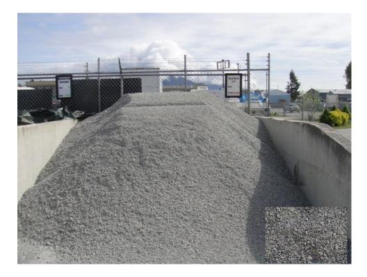
$\frac{3}{4}$ " crushed gravel is a mixture of sand and rock that is best used as packing gravel for underneath asphalt, concrete, driveways, pot holes, garage pads and paving stones. It is also known as  $\frac{3}{4}$ " crush, road crush or road base.
