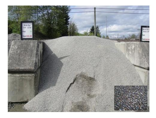
1/8" - 3/16" washed rock is used for landscaping, pipe bedding, mixing in concrete, and as aquarium material. It is also known as pea gravel.
