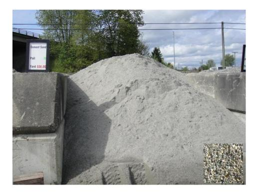
CEMENT SAND is coarser sand used for mixing concrete, loosening up soils in gardens and flowerbeds, and also underneath paving stones.
