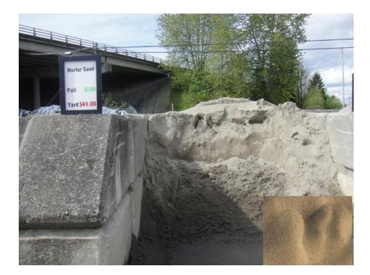
MORTAR SAND is fine mortar sand that can be used for brick laying, masonry work, stucco work, for filling the joints in and around paving stones, and also as play sand. Other names include garden sand, mortar sand, and masonry sand.
