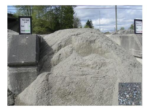
Concrete aggregate mix is three parts 10-28 mm washed rock and 2 parts 5 mm sand. Add Portland cement to make your own concrete.
